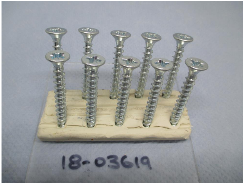
FIG 1: The photograph is showing the condition of the Timco Solo Woodscrew Samples prior to salt spray test
