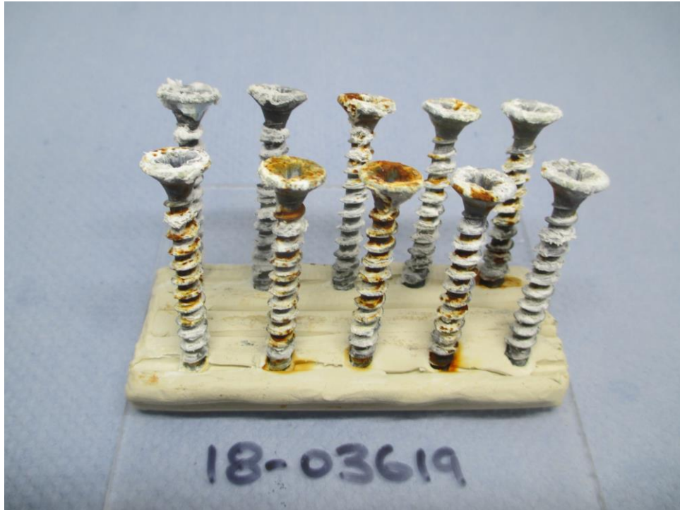
FIG 3: The photograph is showing the condition of the Timco Solo Woodscrew Samples after 120 hours salt spray test
