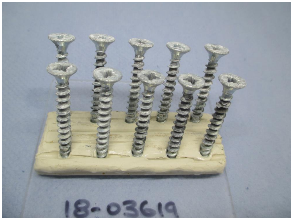
FIG 2: The photograph is showing the condition of the Timco Solo Woodscrew Samples after 24 hours salt spray test
